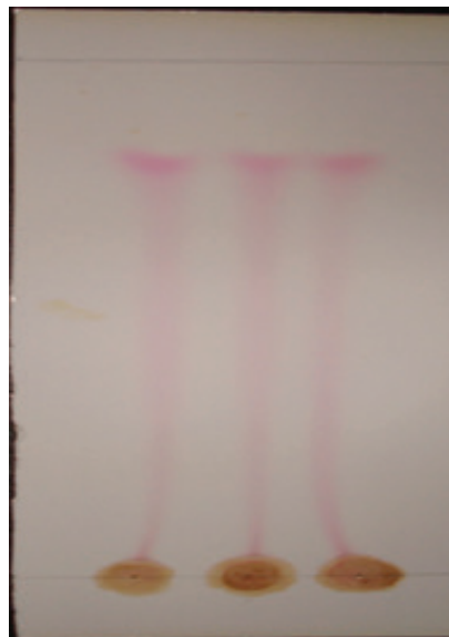
Figure 1: Separation and detection of prodigiosin pigment (Purified) from S. marcescens SKT14 isolate using thin layer chromatography (TLC).
