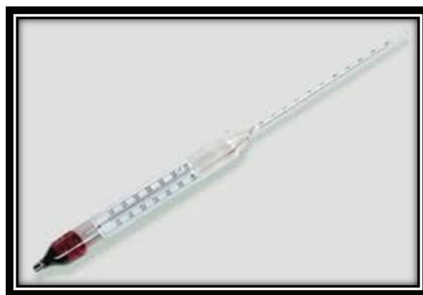
Fig.1: The specific gravity of acetone and the level of dehydration monitor by acetometer
