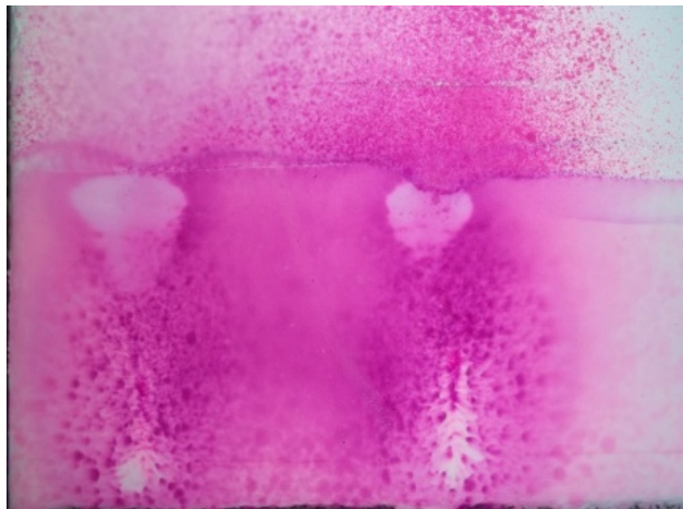
Figure 2: White spots visualized after spraying with Rhodamine B as spray reagent, by using Benzene: Acetone: Ammonia 50:30:20 as solvent system for detection of Cypermethrin by TLC
