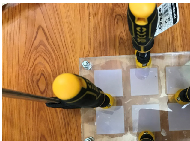
Figure 2: Mold tightened with nuts and G-clamps.
