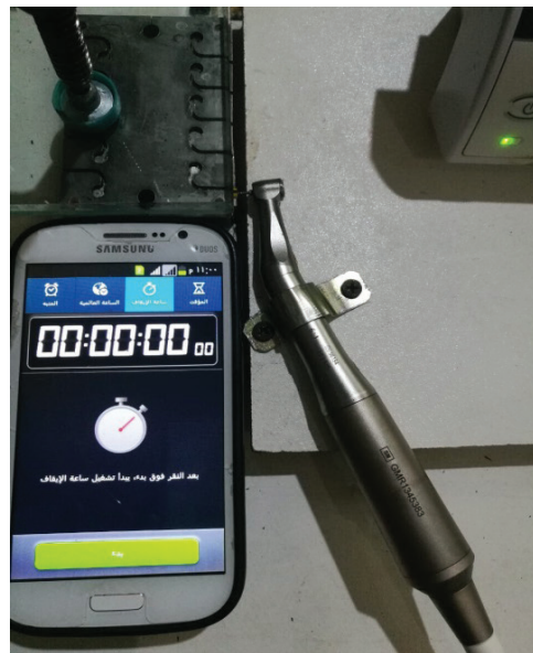
Figure 2: Cyclic fatigue testing device.
