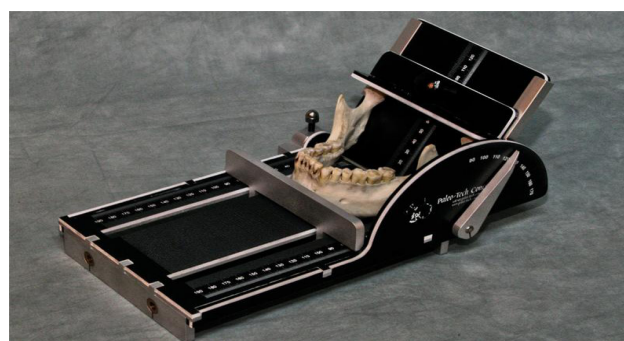
Fig. 4: Mandibulometer, a specific apparatus, being used for measuring mandibular angle
